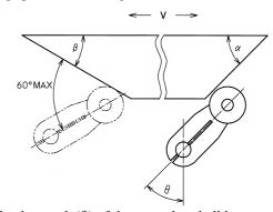
The dog angle( $\beta$ ) of the rear edge shall be set within a range of 15° to 30° to avoid the double action of lever.
