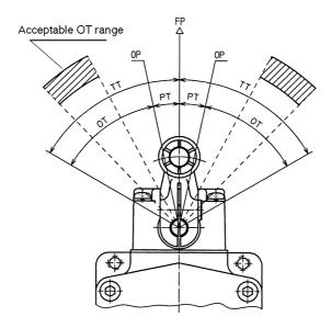
(2) To ensure stable operation, overtravel, defined as any movement of the limit switch lever after operation, must be adjusted within 30 to 70% of the specification value (minimum value).
