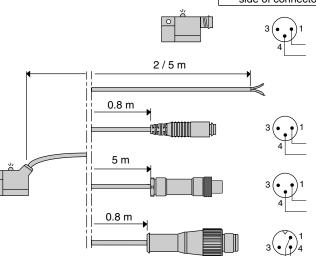
Lead outlet Ø 3 mm with stripped ends,
